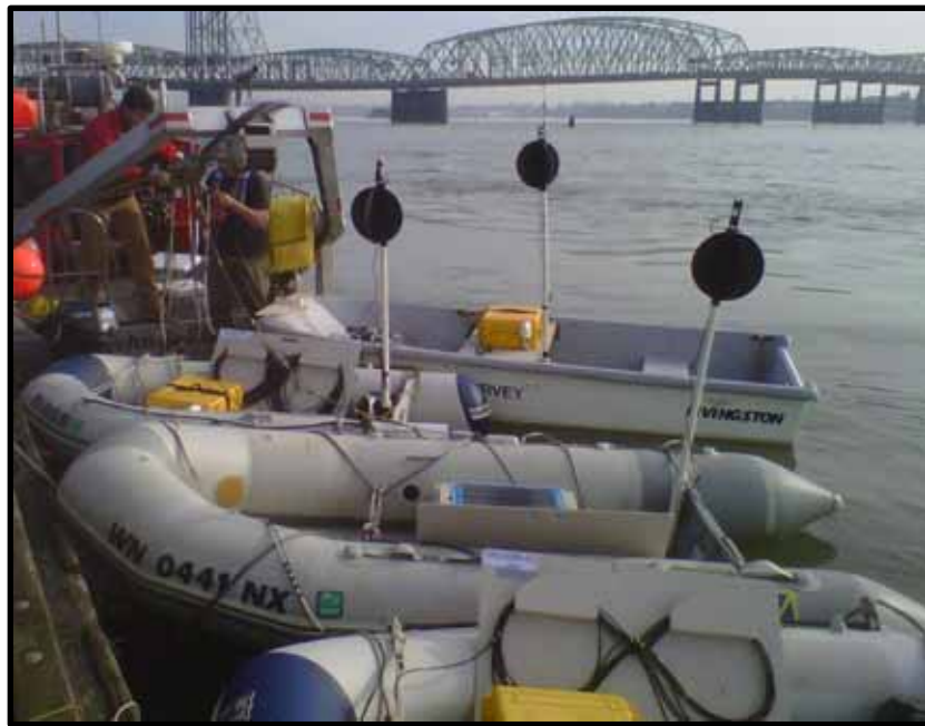
FIGURE 2-3. UNMANNED REMOTELY OPERATED SOUND MONITORING PLATFORMS
